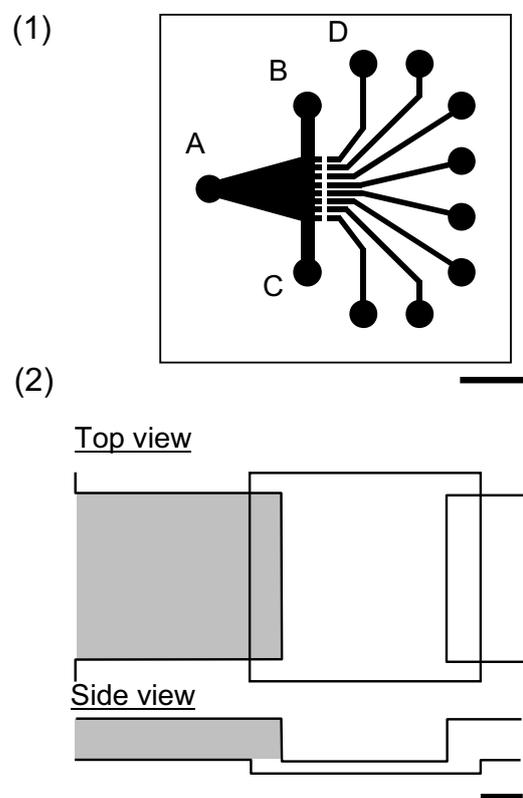
Fig. 2 Structure of the microfluidic device. (1) Design of the device; A: Inlet port, B, C: Side port, D: Outlet port; (2) top and side view of cultivation chamber. Gray area is a cultivation chamber. The volume of the chamber is 20 nL. Each scale bar indicates (1) 5 mm and (2) 100  $\mu\text{m}$ , respectively.
