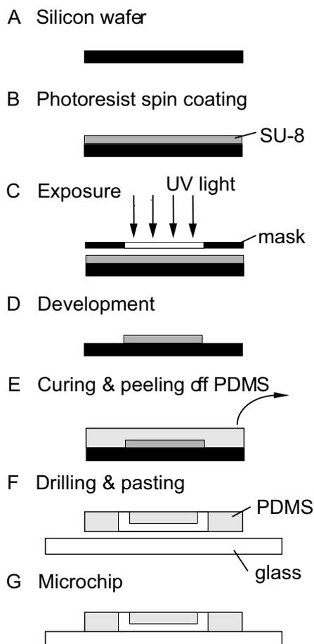
Fig. 1 Fabrication of polydimethylsiloxane (PDMS) microreactor.
