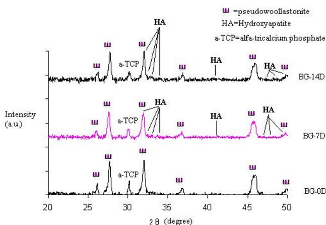
**Fig. 1** XRD patterns of samples BG-0D, BG-7D and BG-14D.
