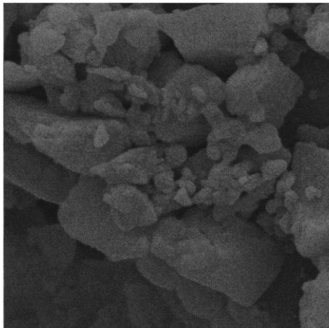
Fig. 3 SEM of bioactive glass before soaking in SBF (BG-0D).
