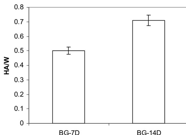
**Fig. 2** Ratio of hydroxyapatite to pseudowollastonite for the samples BG-7D and BG-14D. Values represent mean  $\pm$  Standard Error (SE).  $n = 3$ .
