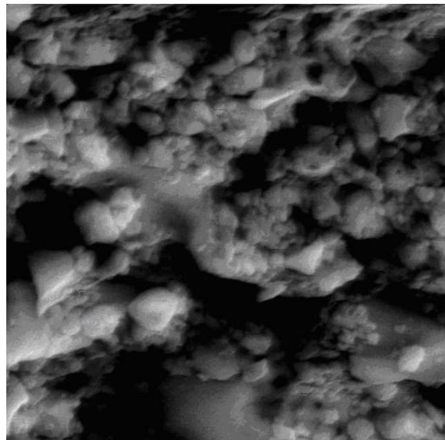
Fig. 4 SEM of bioactive glass after soaking in SBF for 14 days (BG-14D).
