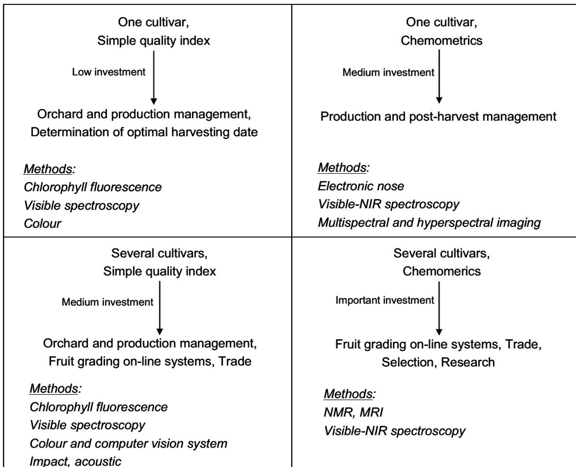
Fig. 1 Schematic diagram of classification of non-destructive methods.
