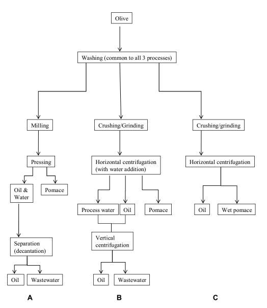
Fig. 1 Flow diagram of the three olive oil extraction processes. (A) Traditional method, (B) three-phase extraction process, (C) two-phase extraction process
