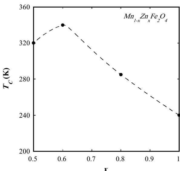
Fig. 5 Curie temperature,  $T_C$ , as a function of the Zn concentration,  $x$  for all the  $Mn_{1-x}Zn_xFe_2O_4$  nanoparticles.
