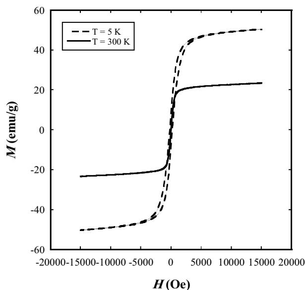
**Fig. 2** Magnetization hysteresis loops for Mn<sub>1-x</sub>Zn<sub>x</sub>Fe<sub>2</sub>O<sub>4</sub> nanoparticles. x = 0.5 at 5 K and 300 K.
