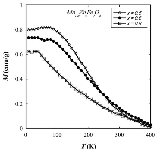
Fig. 4 Temperature dependence of magnetization,  $M(T)$ , for  $Mn_{1-x}Zn_xFe_2O_4$  nanoparticles.  $x = 0.5, 0.6$ , and  $0.8$ .
