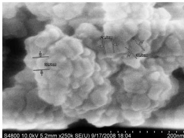
**Fig. 1** SEM image of Mn<sub>1-x</sub>Zn<sub>x</sub>Fe<sub>2</sub>O<sub>4</sub> nanoparticles. x = 0.5.
