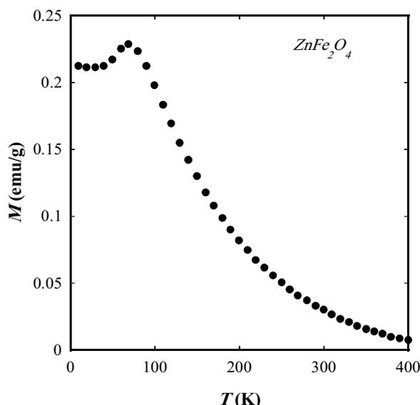
**Fig. 3** Temperature dependence of magnetization, M(T), for ZnFe<sub>2</sub>O<sub>4</sub> nanoparticles.
